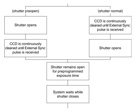
Figure 19. Continuous Cleans Operation Flowchart
